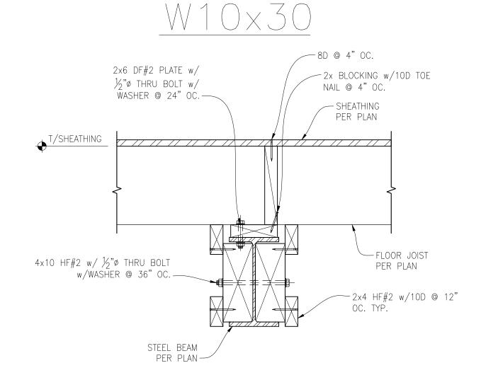
DROPPED STEEL BEAM FLOOR JOIST CONNECTION SCALE:  $1\frac{1}{2}$ " = 1'-0"
