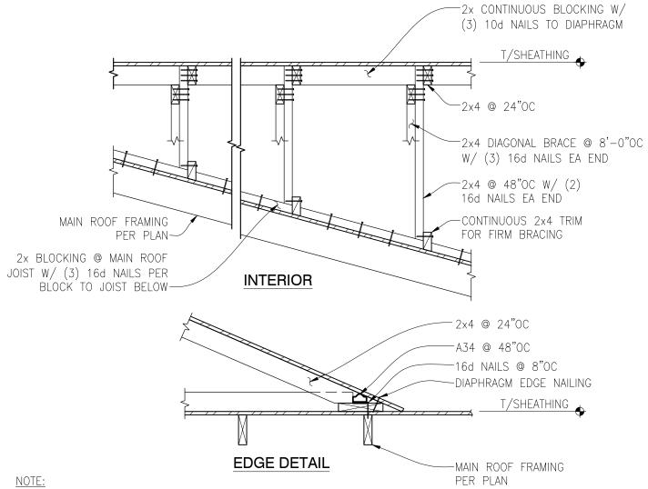
VENTILATION MAY BE REQUIRED AT BLOCKING. VERIFY METHOD WITH ENGINEER PRIOR TO CONSTRUCTION.
