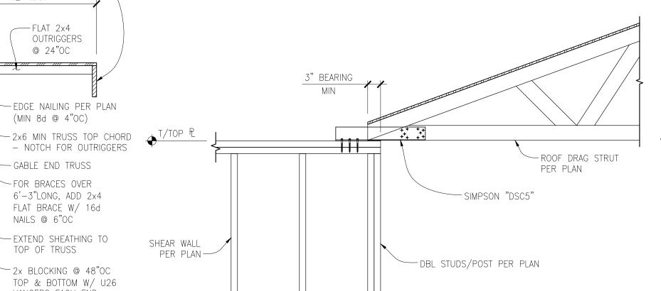
ROOF DRAG STRUT TO SHEAR WALL CONNECTION / SCALE:  $\frac{3}{4}$ " = 1'-0"
