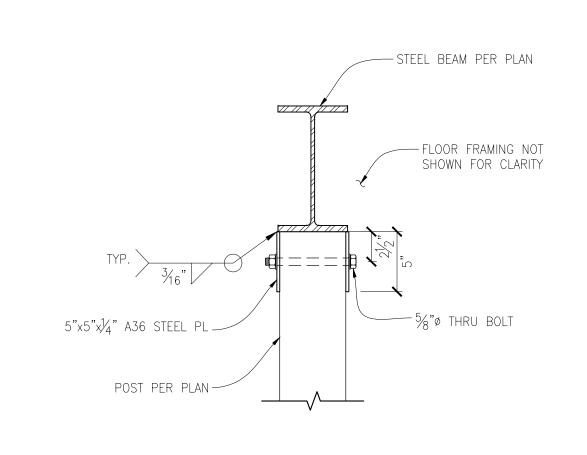
WIDE FLANGE BEAM TO WOOD POST CONNECTION SCALE:  $1\frac{1}{2}$ " = 1'-0"
