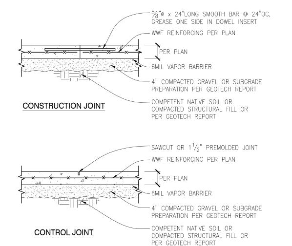
1. FOR CONSTRUCTION OR CONTROL JOINT LOCATIONS REFERENCE FOUNDATION/SLAB PLAN 2. USE "SOFTCUT SAW" AS SOON AS POSSIBLE WITHOUT CAUSING RAVELING OF CONCRETE EDGES.
