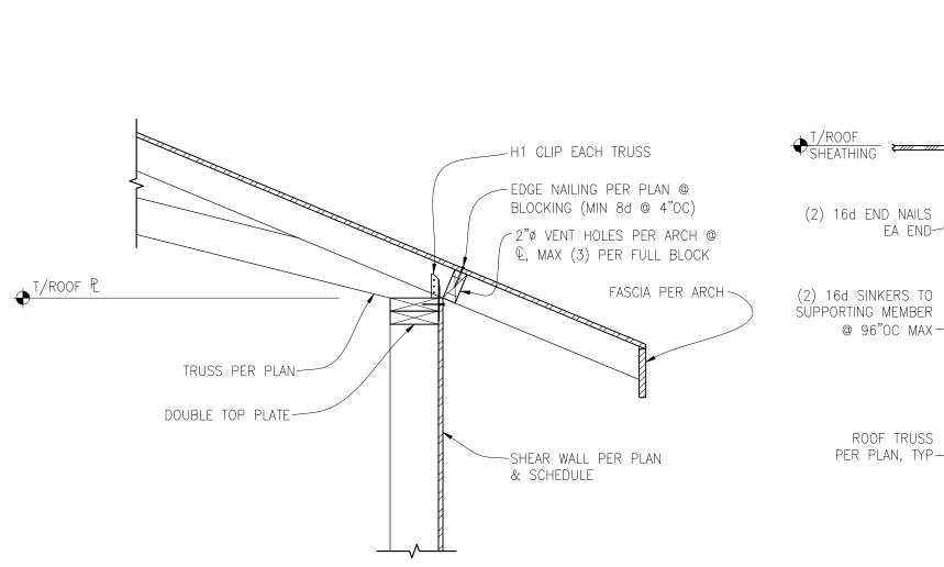
**EXTERIOR SHEAR WALL** PERPENDICULAR TO ROOF TRUSS SCALE: 1" = 1'-0"
